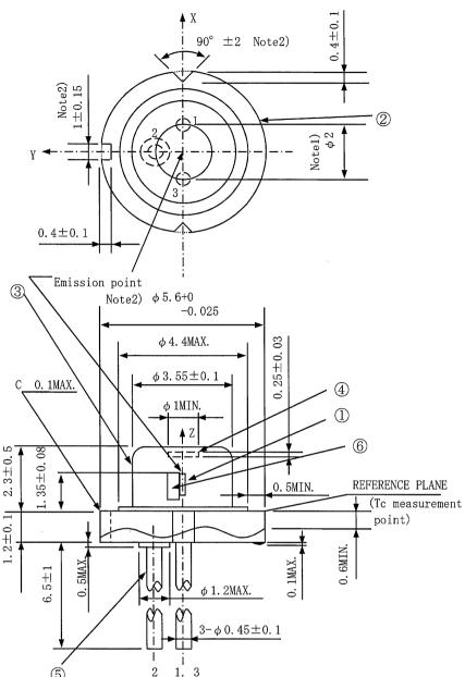
Enlarged drawing around the emission point Emission point  $0 \pm 0.08$  $0 \pm 0.08$
