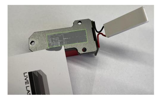
If your Sparrow module does not include a TEC, use the included M3 screws to bolt the module to your heatsink. Start turning the screws but before the tightening, press the module onto the heatsink while applying a twisting motion. The motion helps to spread the paste evenly while squeezing out excess paste. Tighten the screws fully.
