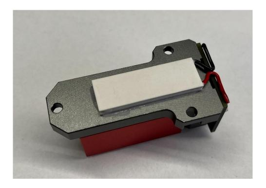
The next step includes spreading the remaining half of the thermal paste on the surface of the TEC. Use the same barleycorn sized amount and spread it like explained before.
